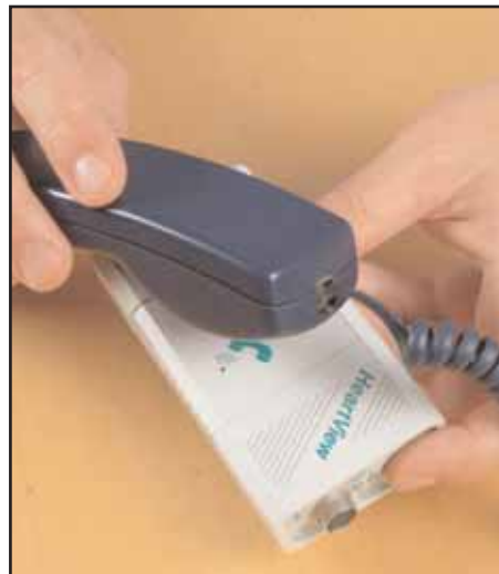
Figure 3. Acoustic transmission of ECG via phone
